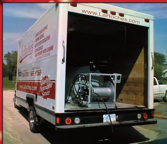
Custom Diesel Powered 18 gpm, 4000 psi in a customer's Van Body Truck
