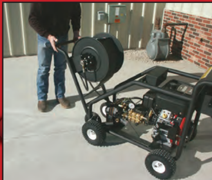
(SW Series) Remove the reel cart and position by drain.
