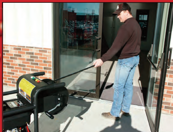
(SW Series) Connect the reel feed hose.
