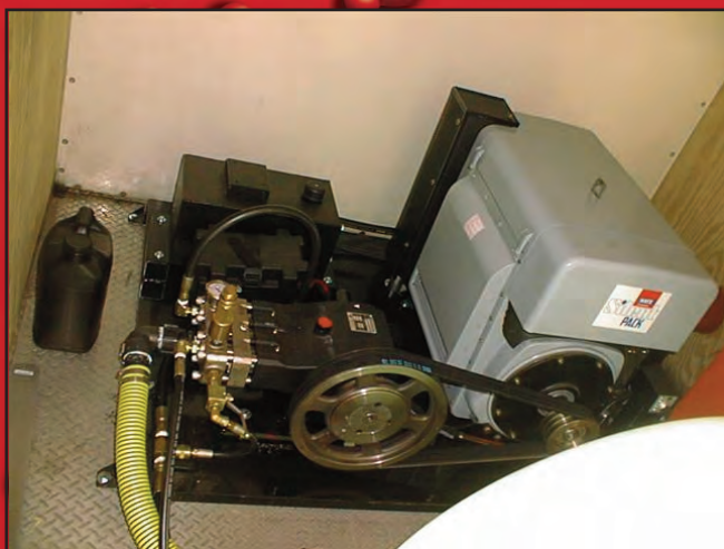
18 gpm, 4000 psi, Hatz Quiet Pack skid.
