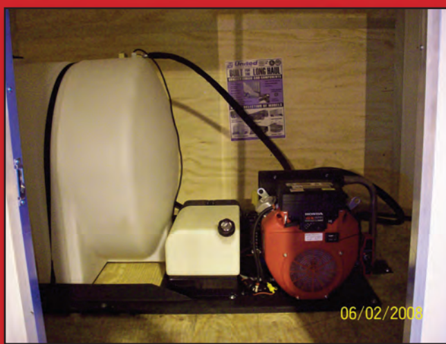
11.5 gpm, 2500 PSI, 325 gallon water tank and hot water option mounted in a customer's enclosed trailer.
